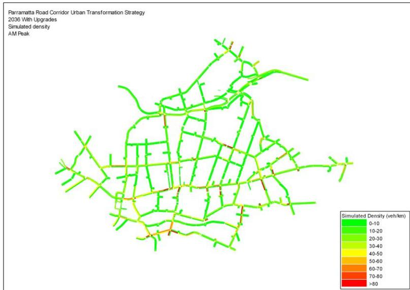
Figure 7-11 Simulated density – 2036 With Upgrades (AM Peak)
