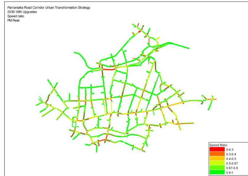
Figure 7-16 Speed ratio – 2036 With Upgrades (PM Peak)
