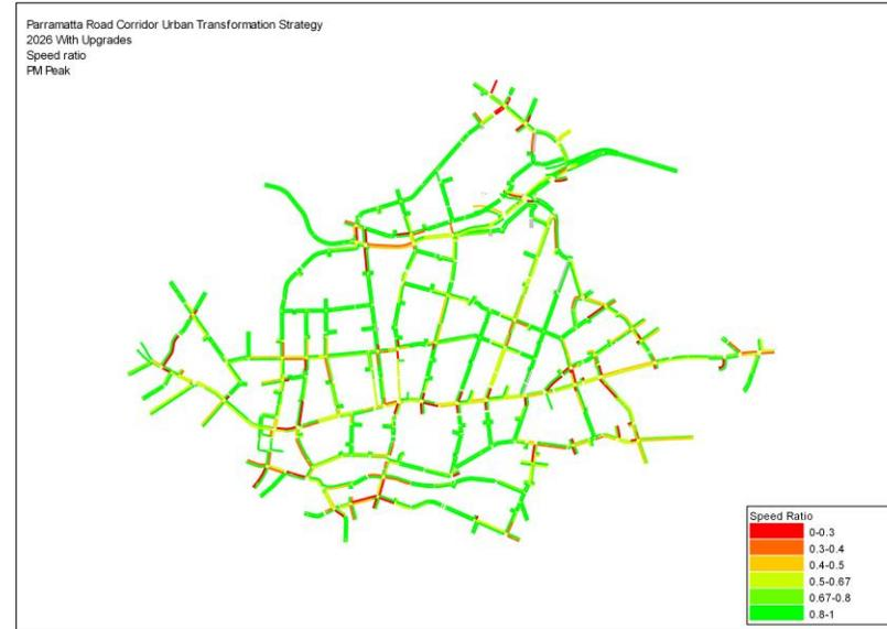
Figure 7-14 Speed ratio – 2026 With Upgrades (PM Peak)
