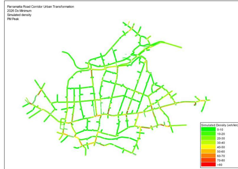
Figure 6-10 Simulated density – 2026 Do Minimum (PM Peak)
