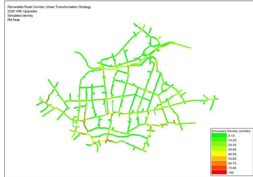
Figure 7-10 Simulated density – 2026 With Upgrades (PM Peak)
