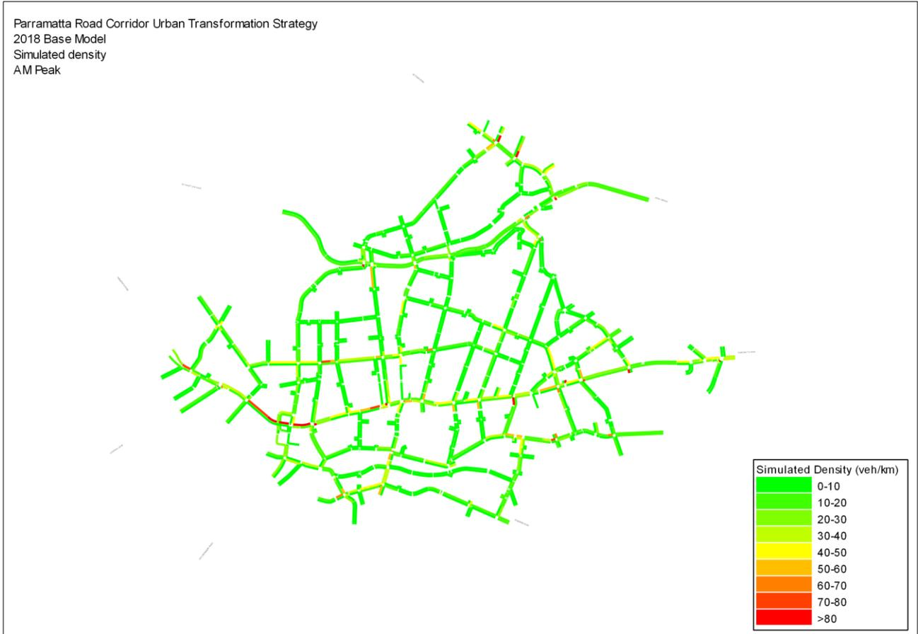
Figure 5-5 Simulated density – Base Model (AM Peak)
