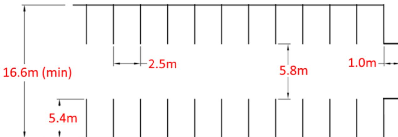
This design gives a minimum floorplate dimension of 16.6m, below which parking cannot be supplied in an efficient manner. For example, a single-sided aisle requires approximately 40% more area per bay, with an equivalent cost increase.
