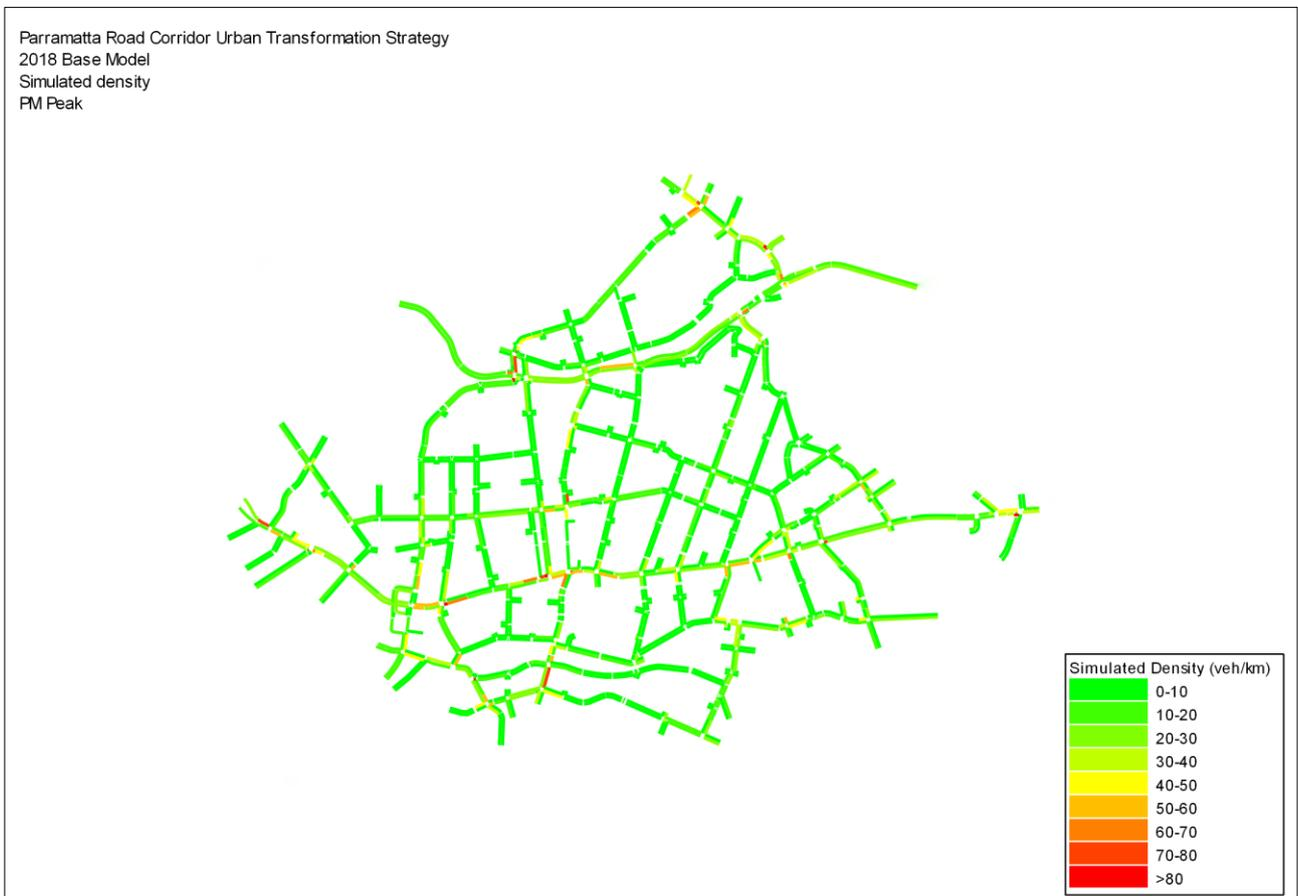
Figure 5-6 Simulated density – Base Model (PM Peak)
