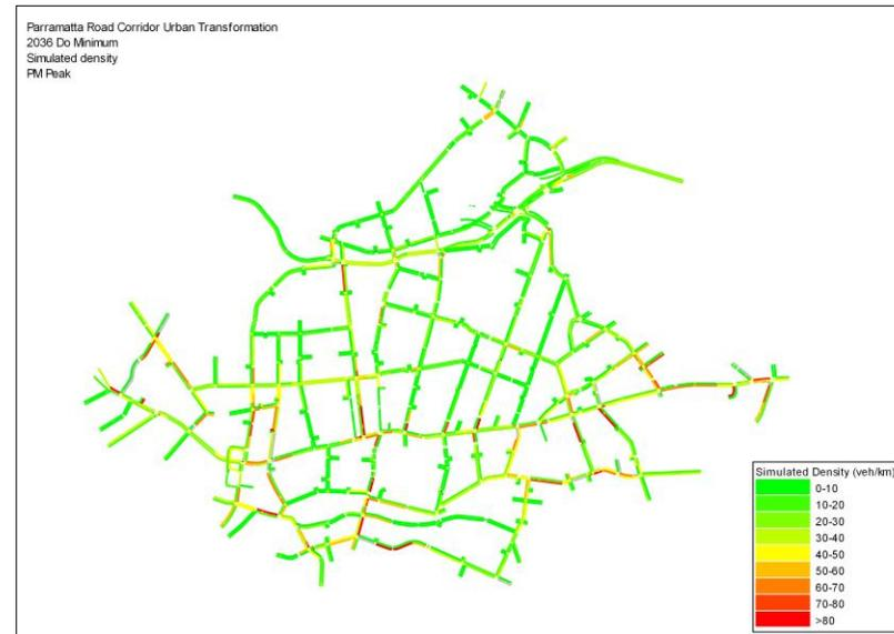
Figure 6-12 Simulated density – 2036 Do Minimum (PM Peak)
