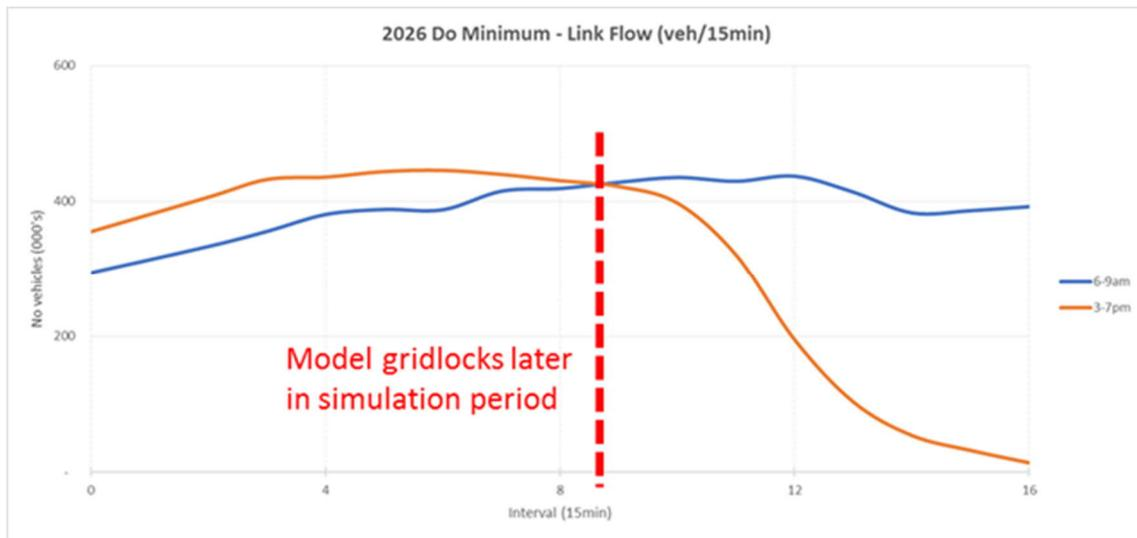
**Figure 1 – Example of identification of network gridlock**
