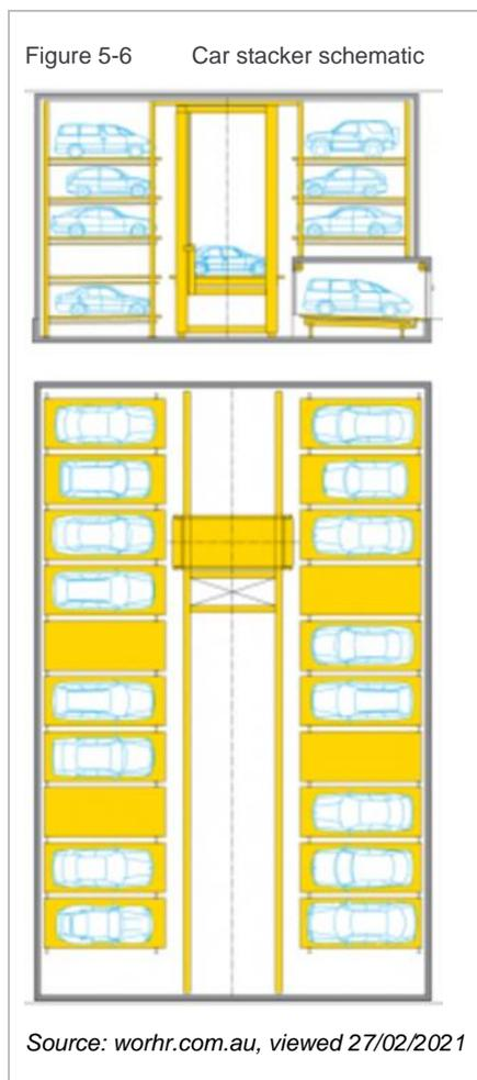
Despite some issues, car stackers may present the best option for on-site car parking where lot geometry does not support efficient car parking. Car stackers installations should be accompanied by supportive documentation that details any limitations on vehicle use, how spaces will be allocated, the operational framework, queuing projections and mitigation measures.
